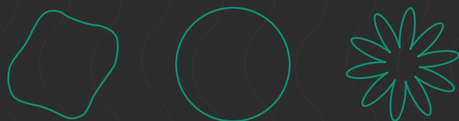
Figure 1: Among curves of a fixed length, the circle encloses the largest area.
