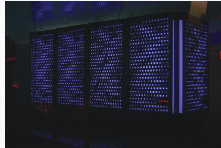
Example of an Anton supercomputer. Designed and built by D.E. Shaw Research, the third-generation Anton supercomputer will simulate biomolecules roughly 100 times faster than general-purpose supercomputers.
